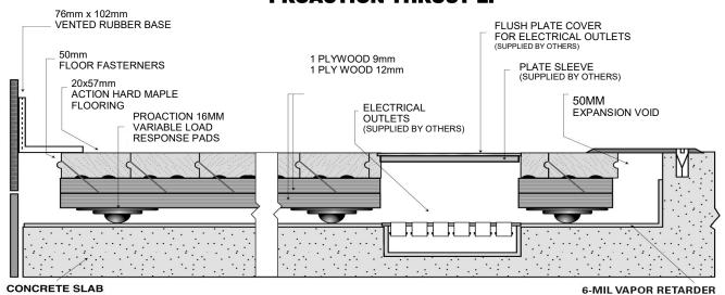
This flooring system consists of 32 natural rubber pads per 2.88m2, 2 layers of plywood and 20mm thick solid American Maple Flooring. The floor is finished on site using two coats of oil based timber seal, hand painted court lines and two coats of a sports floor finish, which provides the right amount of slip Resistance.
